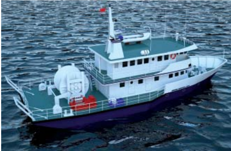
Artist's impression of the Tanganyika Explorer post conversion to a 2D seismic vessel
